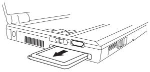
Sample removing a PC Card
